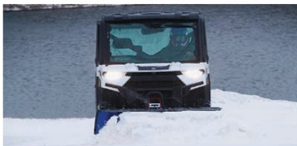
PLOW IS AUTOMATICALLY LOWERED WHEN SHIFTING INTO LOW
