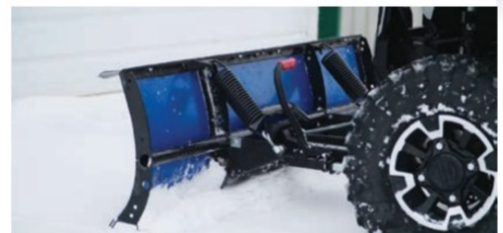
BACK DRAG MODE ALLOWS FOR PULLING SNOW AWAY FROM BUILDINGS
