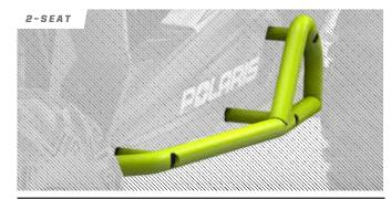
**4.45 CM DIAMETER** STEEL TUBE CONSTRUCTION
